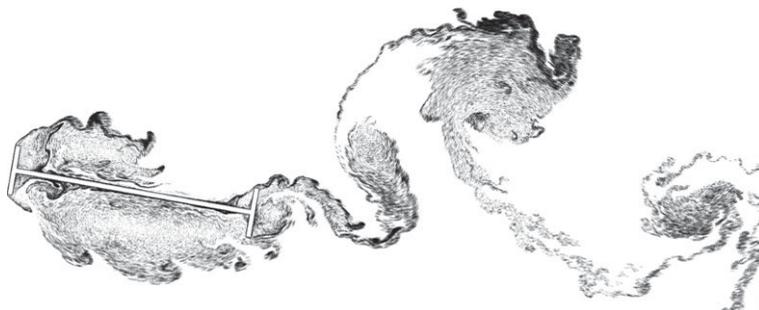
**Figure 3.** A vortex particle simulation of the first Tacoma Narrows Bridge undergoing large-amplitude prescribed periodic torsional motions. The figure, produced using Morgenthal's VXFLOW [24], illustrates Larsen's vortex drift hypothesis, with large leading-edge vortices drifting across the deck, above and below, inducing periodic forces on the leeward portions of the deck.
