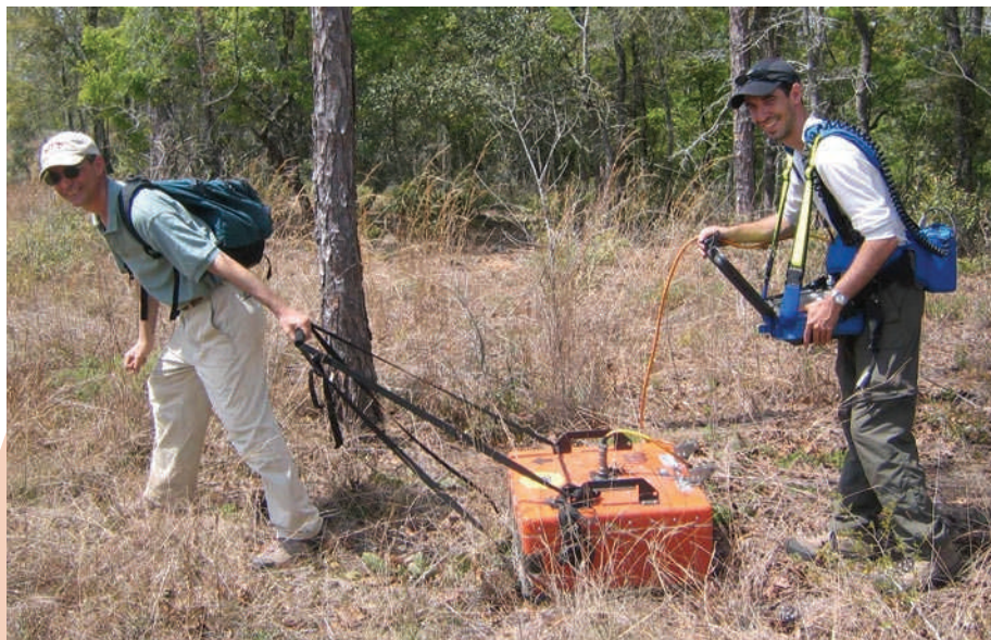
Daniel Rothman (left) and Kyle Straub during an early attempt to obtain ground-penetrating radar data to map the water table.
